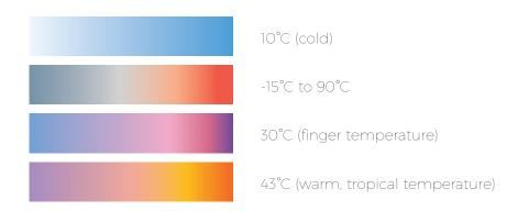
Thermochromic pigments are made up of microcapsules or microspheres containing a colourant that is sensitive to temperature. These microcapsules are typically mixed into paints, inks, or coatings, allowing them to be applied to various surfaces.
